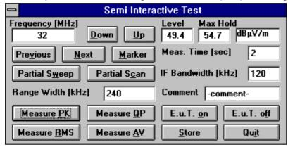
By clicking Down and Up the arbitrarily editable frequency will be decreased and increased by the step size defined in the scan table. If the test is based on a frequency list or on a measurement result list then with Previous and Next the switch dialogue will to the corresponding frequency. With measurement results the referring positions of the antenna and the EuT can optionally be set. A click on the button Marker will copy the
